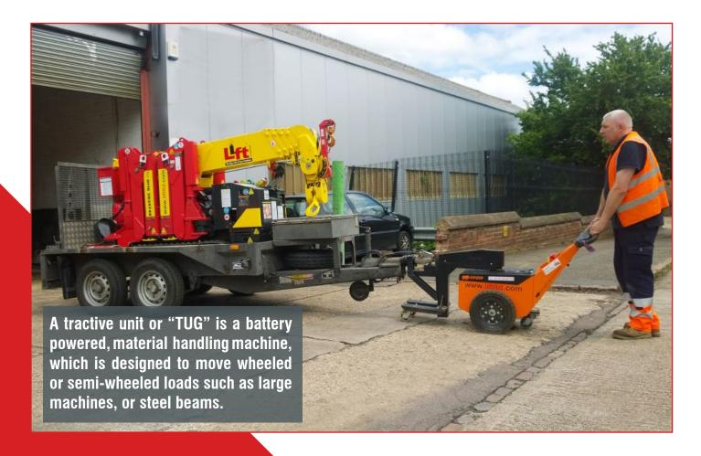
Amongst our wide range of lifting/pulling or moving equipment hire fleet, LIFT offer this exceptional unit to go hand in hand with our spider cranes to address the issue of manual handling heavy loads. Especially when maintaining the finished products quality — the "TUG" will operate under complete control, allowing a steady and controlled movement of a load.
