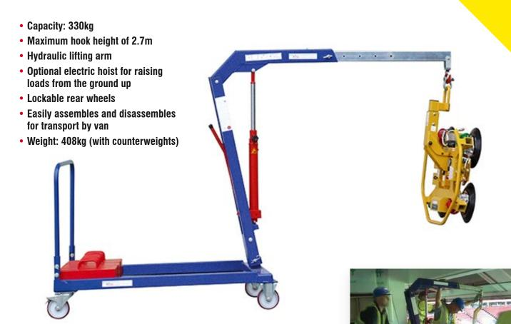
The Glassboy 330 is a versatile counterbalanced floor crane that is a proven best seller thanks to its easy-to-assemble, highly portable frame, and flexibility to assist in a broad range of applications. With the ability to handle loads of up to 330kg and a maximum hook height of 2.7m, the Glassboy 330 is a compact and reliable lifting aid. When combined with a range of below-the-hook devices such as vacuum lifters, it is ideal for shop-front glazing and fitting below overhangs.
