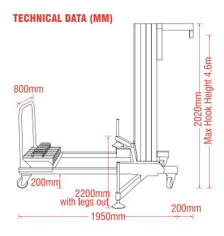
Note 1: Counterweights must be secured before lifting. Note 2: When using fork attachment the load must be centralised and secured.
